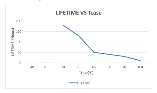
Lifetime ≥ 30,000 hrs. @ 65°C case temperature checked at ambient 50°C refers to lifetime vs. case temperature graph
